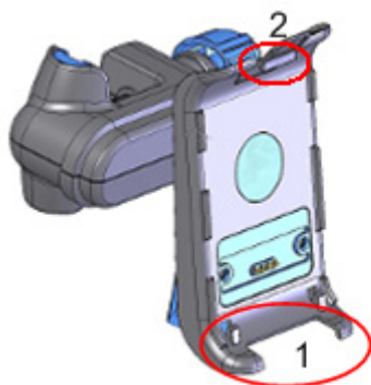
Figure 2.4. Crochets du mini-support
